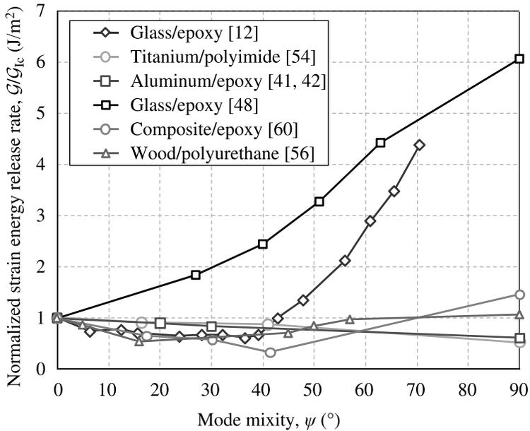
**Figure 7.** Examples of variation of fracture energies as a function of mode mixity for a range of adhesively bonded systems.
