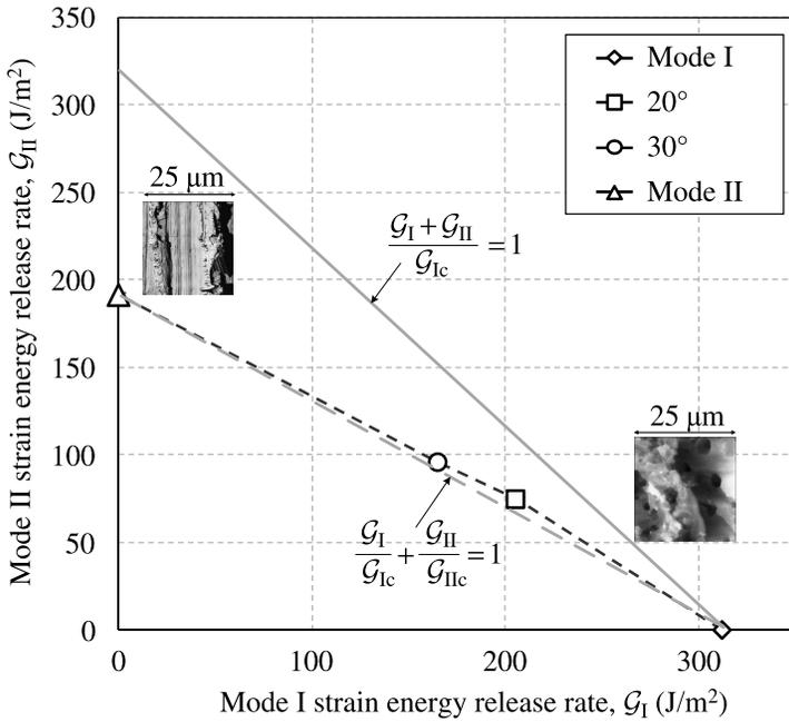
Figure 3. Fracture envelopes for aluminum adherends bonded with a rubber toughened epoxy.
