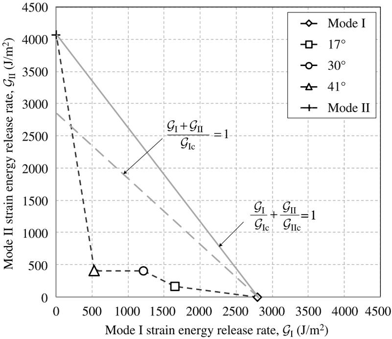
**Figure 6.** Fracture envelopes for composite adherends bonded with a 2-part commercially available epoxy.
