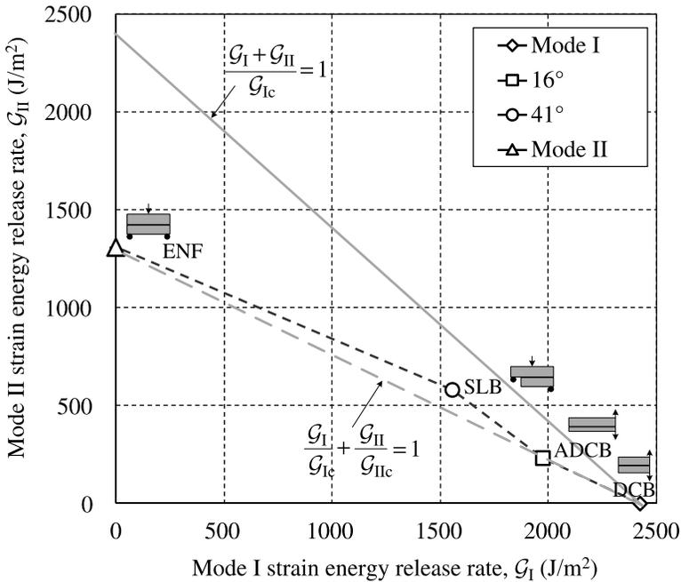
**Figure 2.** Fracture envelopes for titanium adherends bonded with a polyimide adhesive.
