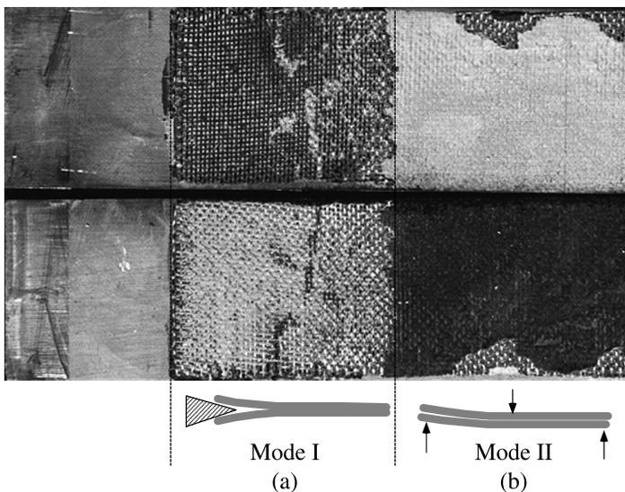
**Figure 1.** Locus of failure for (a) mode I and (b) mode II loaded regions of titanium adherends bonded with a polyimide adhesive film supported on a fiberglass scrim cloth.
