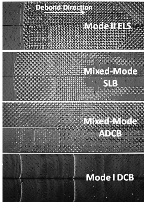
**Figure 5.** Illustration of locus of failure resulting from a range of applied fracture modes for composite adherends bonded with epoxy adhesive.
