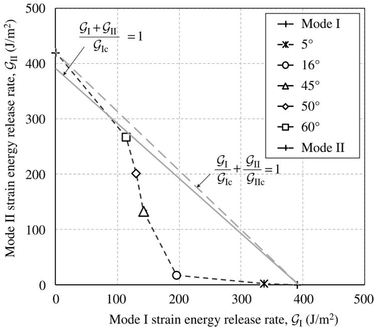
Figure 4. Fracture envelopes for southern yellow pine (*pinus spp*) adherends bonded with a polyurethane adhesive.
