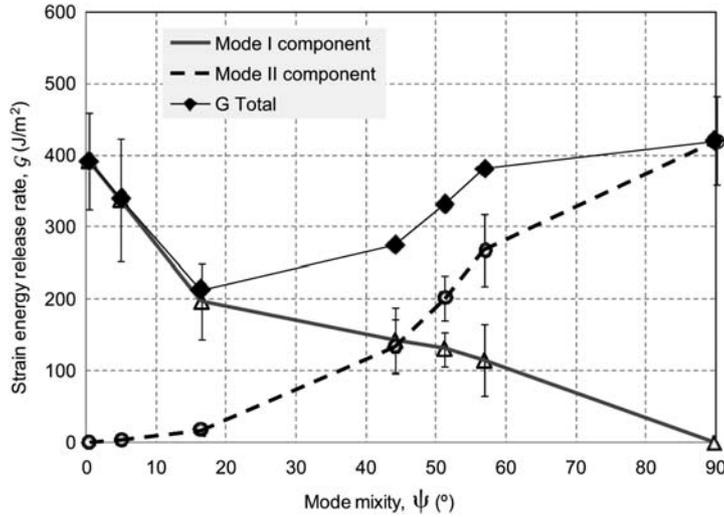
**Figure 5** Variation of total value of strain energy release rate as well as mode I and mode II components as a function of mode mixity. Error bars indicate  $\pm 1$  SD.
