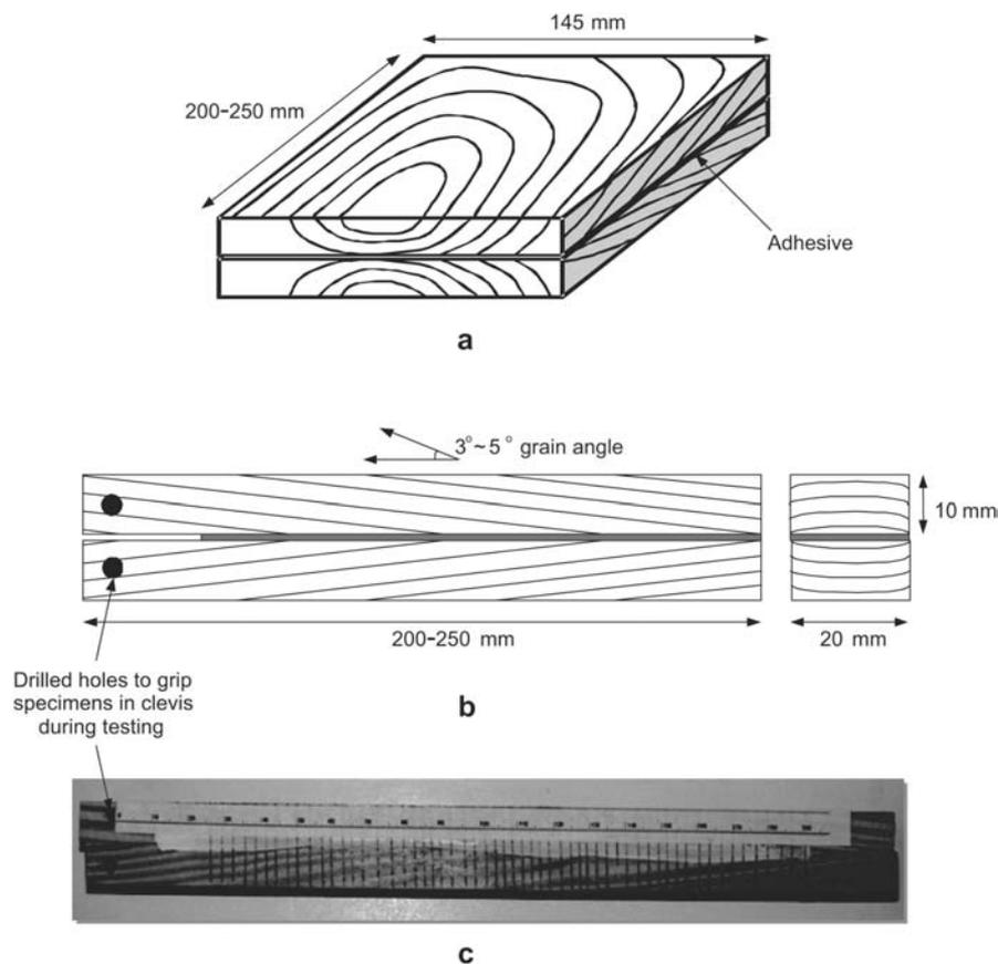
**Figure 2** Double cantilever beam (DCB) sample preparation method: (a) two wooden laminates bonded together with polyurethane adhesive, (b) illustration of a typical DCB specimen with dimensions and grain angle obtained from cutting the bonded wood laminate into 4 or 5 specimens, (c) DCB sample painted with white correction fluid and marked with parallel lines along with the attached paper scale.
