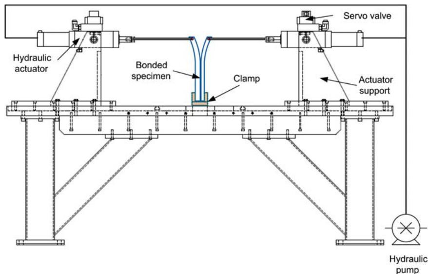
**Figure 1** Schematic illustration of the dual actuator load frame.
