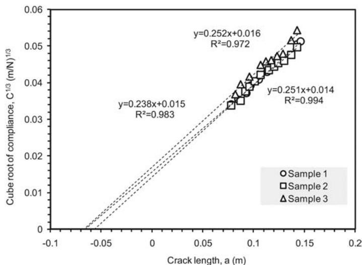
Figure 4 Cube root of compliance versus crack length for wood specimens tested under mode I configurations.
