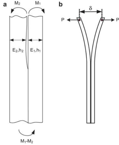
**Figure 3** Double cantilever beam (DCB) specimen (a) loaded with arbitrary bending moments and (b) loaded under mode I configuration.
