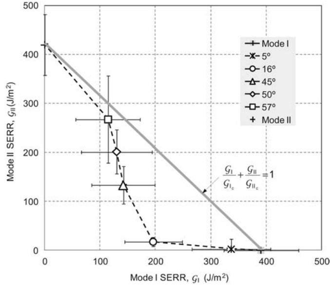
**Figure 6** Mixed mode fracture envelope of southern yellow pine (*Pinus* spp.) bonded with polyurethane adhesive. Error bars indicate  $\pm 1$  SD.
