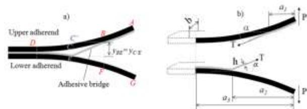
Figure 1. Model of the adhesive bridging problem with geometric parameters, external loads, and tractions exerted by the bridge: a) Schematic of the 2D model; b) Cantilever beam models for the two adherends and definitions of three crack lengths.
