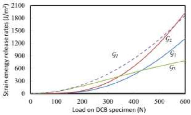
Figure 2. SERR curves for the three crack tips as functions of load  $P$ , with  $a_1 = 50\text{mm}$ ,  $a_2 = 68\text{mm}$ ,  $a_3 = 200\text{mm}$  (Assumes no crack propagation, adhesive with modulus of  $3\text{GPa}$ , thickness of  $0.25\text{mm}$ , bond width of  $25.4\text{mm}$ , aluminum adherends with modulus of  $70\text{GPa}$ , width of  $25.4\text{mm}$ , and thickness of  $12.7\text{mm}$ ).
