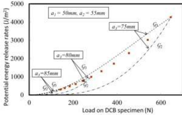
Figure 4. Balance points with different values of  $a_3$  ( $a_1 = 50mm$  and  $a_2 = 55mm$  are fixed).
