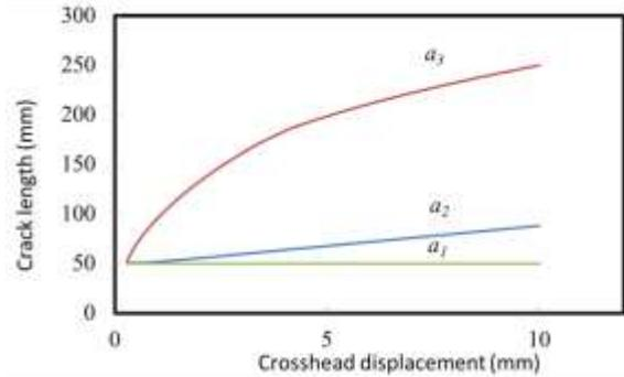
Figure 3. Crack propagation sequences calculated by the 2D model. (The initial crack lengths,  $a_1 = 50\text{mm}$ ,  $a_2 = 51\text{mm}$ , and  $a_3 = 52\text{mm}$  are assumed. Fracture energy is assumed to be  $G_c = 300\text{J}/\text{m}^2$  along the bonded surfaces. The increment in calculation is assumed to be  $0.1\text{mm}$  for all the three crack lengths.)
