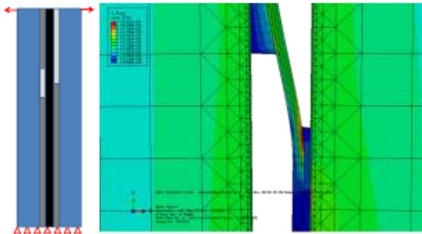
Figure 5. Schematic of geometry, loads, boundary conditions, and result of stress distribution from the simulation of the 2D bridging problem in ABAQUS (The thickness of interfaces shown is only for visualization, and is very small in the calculation).
