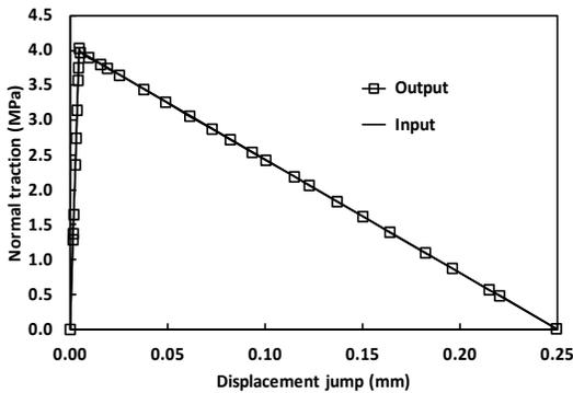
**Figure 2.** Traction separation law for pure mode I
