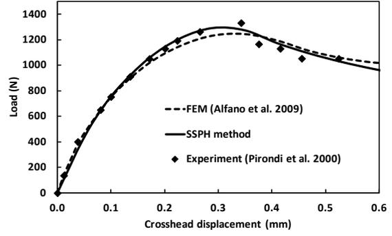
**Figure 3.** Comparison of the numerically computed and experimentally observed load vs. displacement curves.
