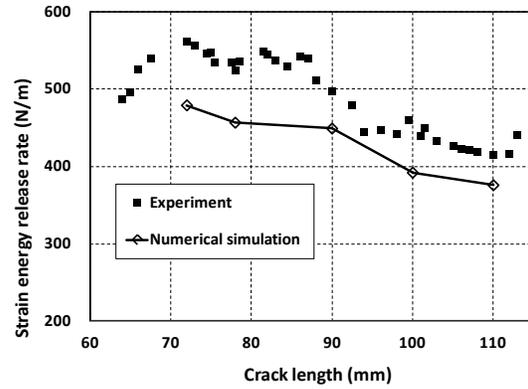
**Figure 7.** Comparison of the computed and the experimental strain energy release rate vs. the crack length for specimen S287.
