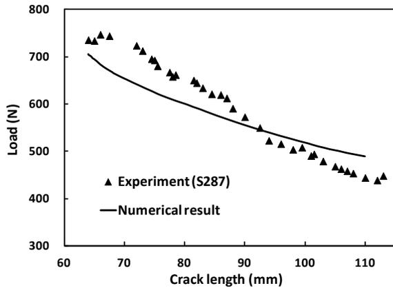
**Figure 6.** Comparison of the computed and the experimental load vs. crack length curve.
