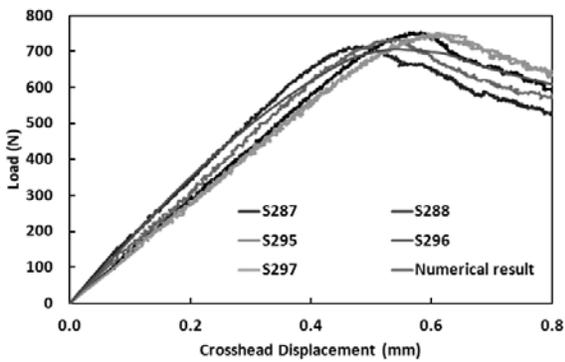
**Figure 5.** Comparison of the computed and experimental (5 specimens) load-displacement curves.
