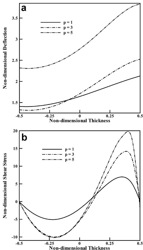
Fig. 9. Effect of the exponent  $p$  on the through-the-thickness variation of a the transverse deflection, and b the transverse shear stress on the section  $x_1 = 125$  mm
