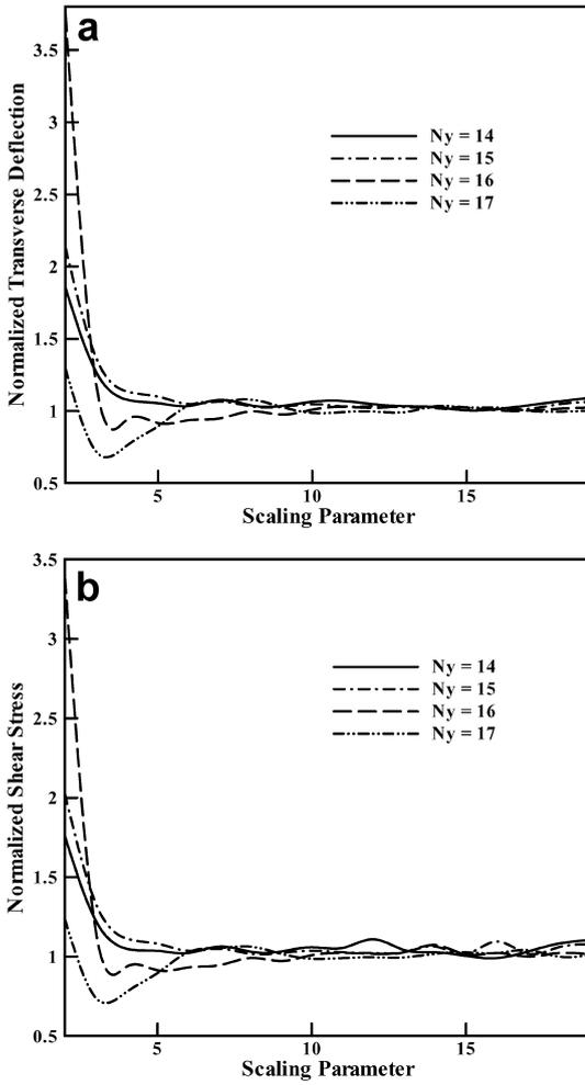
Fig. 7. Convergence of a the deflection at the point  $(L/2, 0)$  and b the transverse shear stress at the point  $(0, 0)$  with the increase in the scaling parameter [ $N_y$  equals the number of uniformly spaced nodes in the  $x_2$ -direction]
