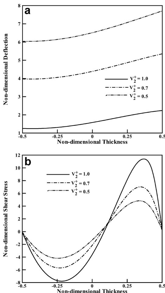
Fig. 10. Effect of  $V_2^+$  (volume fraction of SiC at the top surface) on the through-the-thickness variation of a the transverse deflection, and b the transverse shear stress on the section  $x_1 = L/2$  mm
