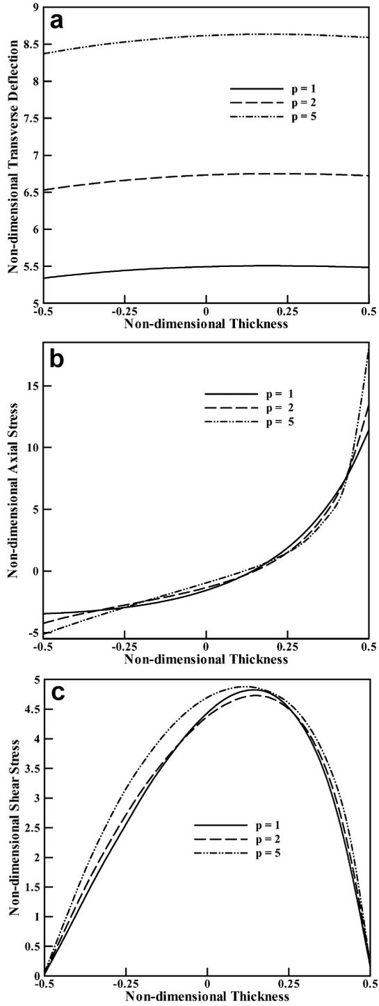
Fig. 4. Effect of the exponent  $p$  on the through-the-thickness variation of a the transverse deflection, b the axial stress, and c the transverse shear stress, on the section  $x_1 = L/2$
