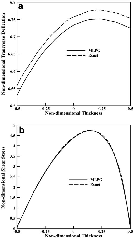
Fig. 3. For the pressure loading, comparison of through-the-thickness variation of a the transverse deflection and b the transverse shear stress at  $x_1 = L/2$  computed by the MLPG method with the analytical solution of Vel and Batra [42]
