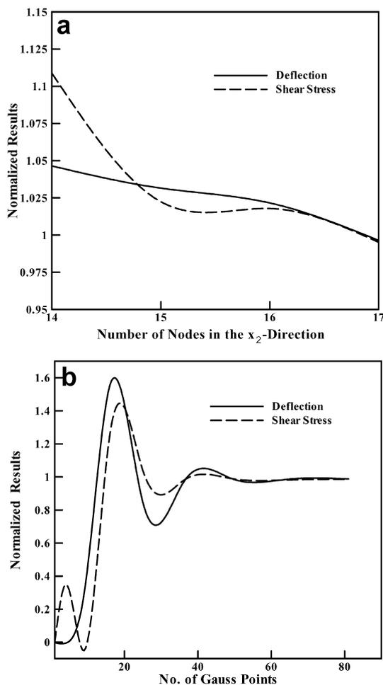
Fig. 6. Convergence of the deflection at the point  $(L/2, 0)$  and the transverse shear stress at the point  $(0, 0)$  with the increase in the number of a nodes in the  $x_2$ -direction, and b Gauss points
