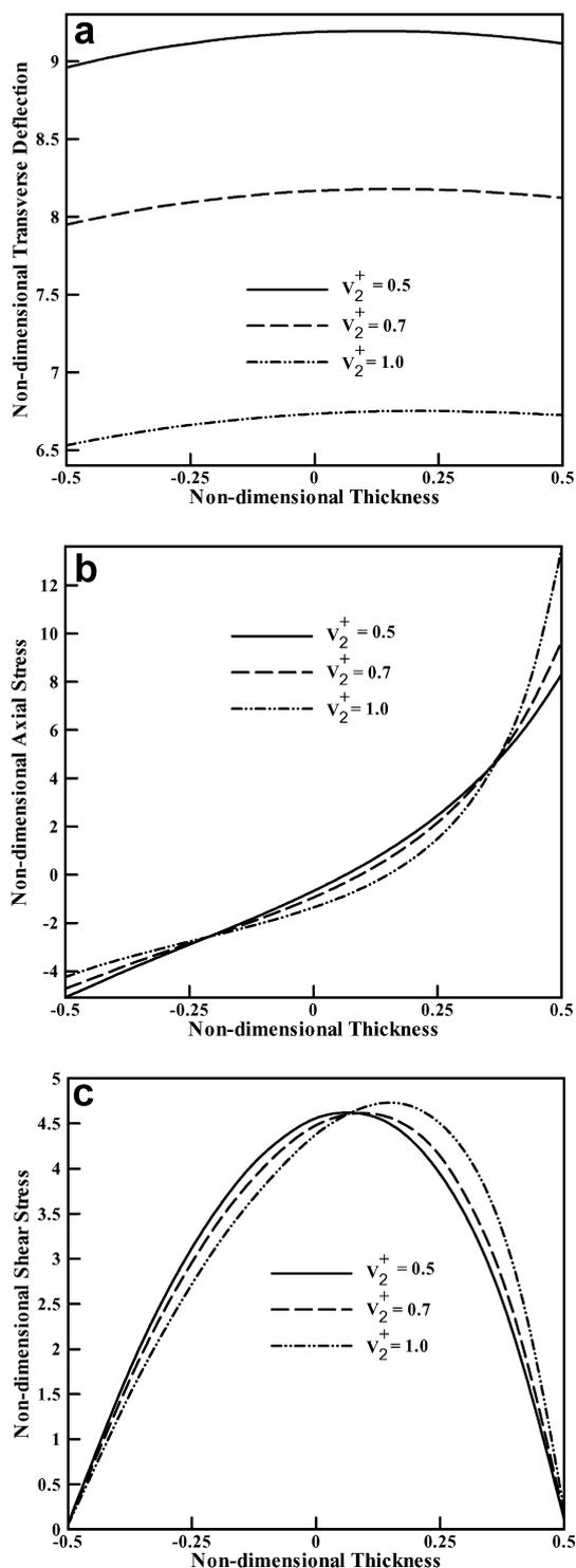
Fig. 5. Effect of  $V_2^+$  (volume fraction of SiC at the top surface) on the through-the-thickness variation of a the transverse deflection, b the axial stress, and c the transverse shear stress, on the section  $x_1 = L/2$
