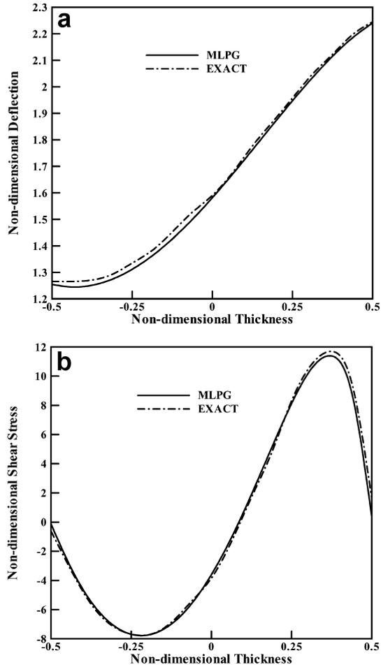
Fig. 8. For the thermal loading, comparison of through-the-thickness variation of a the transverse deflection and b the transverse shear stress at  $x_1 = L/2$  mm computed by the MLPG method with the analytical solution of Vel and Batra [42]
