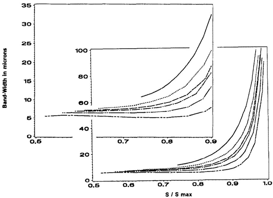
Fig. 7. Dependence of the band width upon  $s_a/s_{max}$ .
