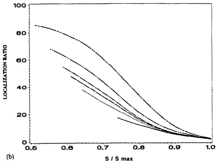
Fig. 6. (a) The shear strain  $\gamma_{loc}$  at the band center vs the nominal strain  $\gamma_{avg}$ . (b) The localization ratio ( $\gamma_{loc}/\gamma_{avg}$ ) vs  $s_a/s_{max}$ .
