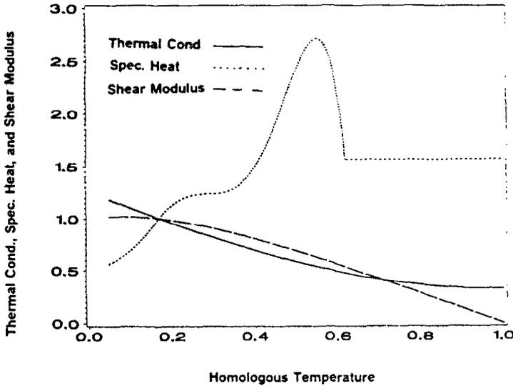
Fig. 1. Dependence of the thermal conductivity, specific heat and shear modulus for the material of the block upon the temperature.
