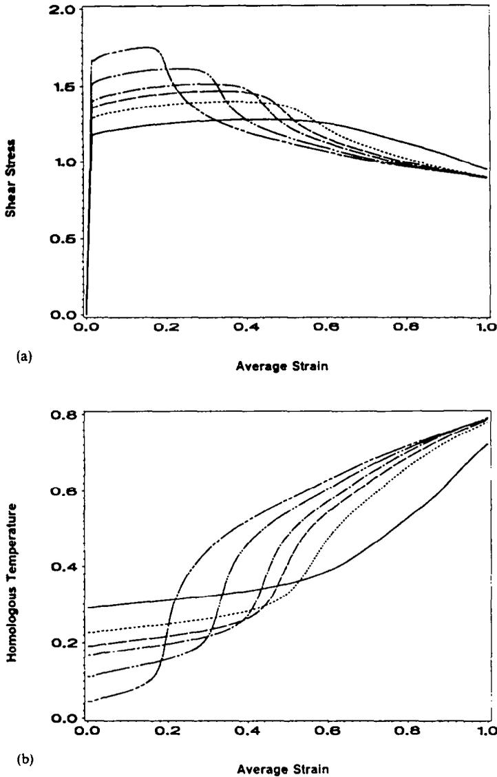
Fig. 2. (a) Average shear stress vs the average shear strain for six different values of the initial temperature of the specimen. (b) Homologous temperature at the center of the specimen vs the average shear strain.
