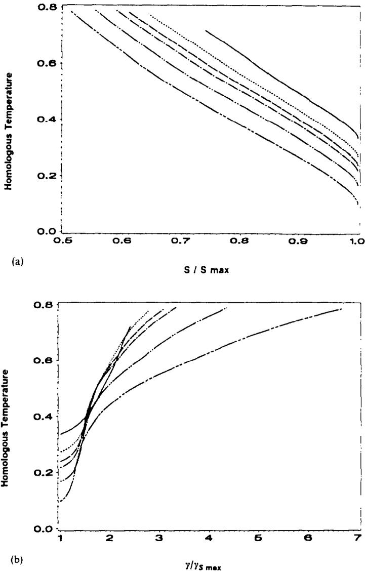
Fig. 3. Evolution of the temperature at the center of the specimen: (a) homologous temperature at the center vs  $s_a/s_{max}$ , (b) homologous temperature at the center of the specimen vs  $\gamma_{avg}/\gamma_a$ . Here  $\gamma_s$  equals the value of  $\gamma_{avg}$  when the average shear stress attains its maximum value.
