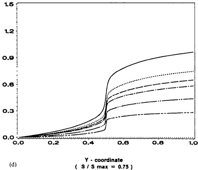
Fig. 5. Deformed shapes of an initial straight line at (a)  $s_a/s_{max} = 1.0$ , (b)  $s_a/s_{max} = 0.95$ , (c)  $s_a/s_{max} = 0.85$ , (d)  $s_a/s_{max} = 0.75$ . The ordinate equals the displacement of a point in the direction of shearing.
