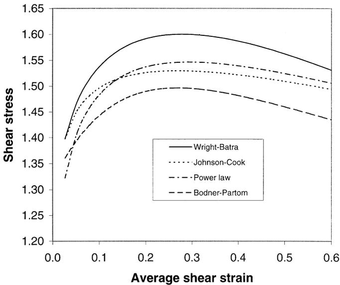
Fig. 1. Shear stress vs. shear strain curves for homogeneous simple shearing deformations of a HY-100 steel at a strain rate of 3300/s.
